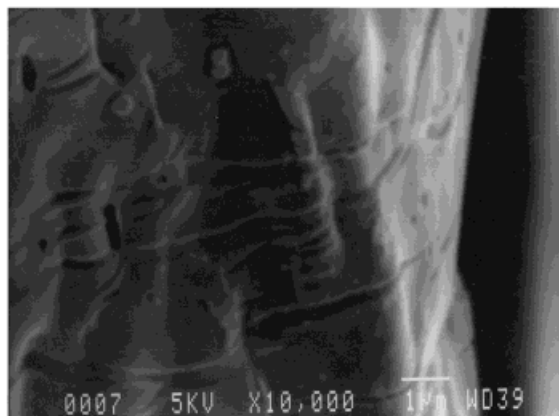
(b) PVC/PVP CROSS SECTION
